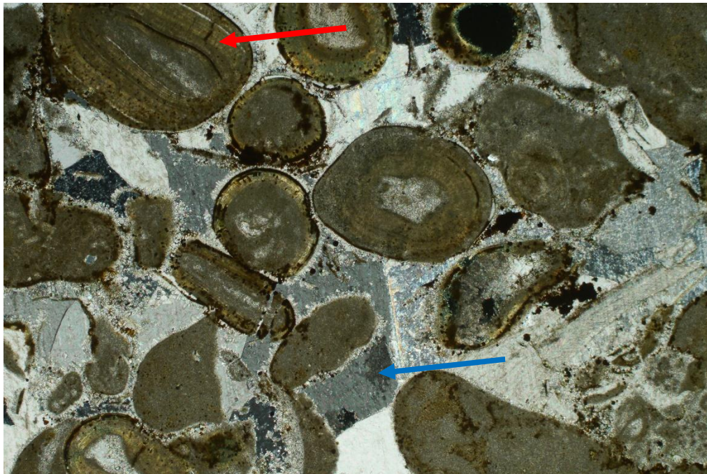
Figure 3. Concentric structure (arrowed red) and sparite cement (arrowed blue). Cross polarised light, magnification x50.
