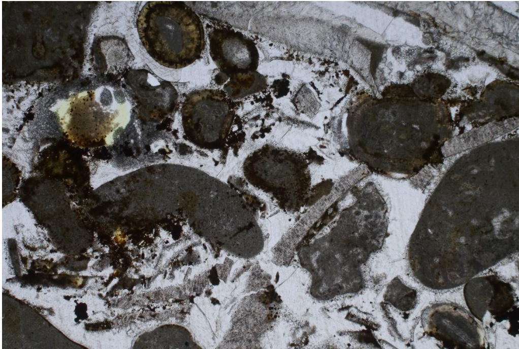
Figure 4. Iron minerals (black in image) producing orange colouration to the surrounding stone. Plane polarised light, magnification x50.
